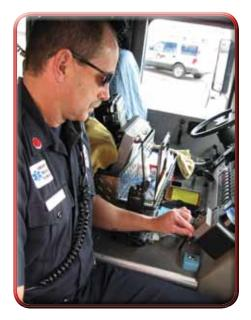
Falcon Fire stores their master key in a KeySecure master key retention unit on the department's apparatus. KeySecure allows every member of the department access to the master key with their own unique PIN code and provides an audit trail showing who gained access to the key and when.
