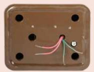
Rear-view of Knox-Box showing tamper switch wires.
